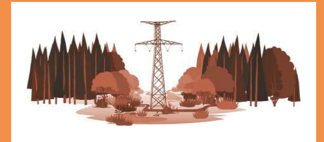
FIGURE 4 USE OF SHORT TREES IN POWER LINE CORRIDORS
