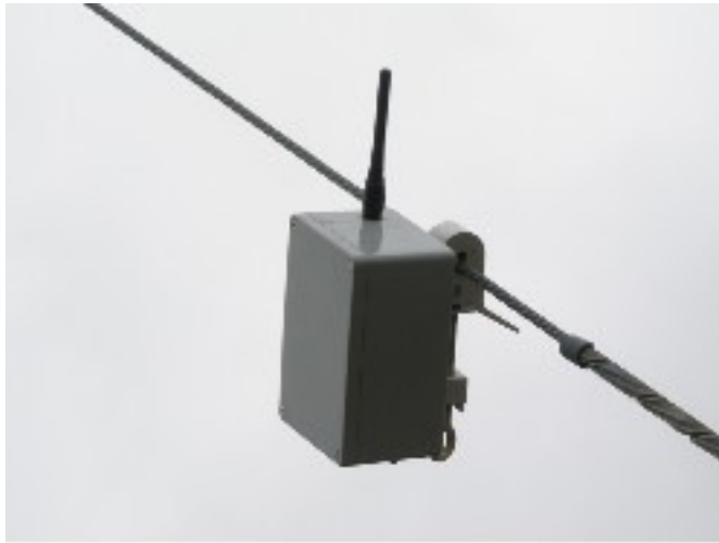
Figure 22. Bird Strike Indicator (BSI) attached to a power line. BSIs are relatively small devices that can be attached to a single wire of a power line and automatically register bird collisions based on the vibration of the wire.
